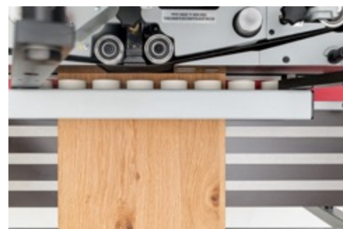
sanding of angular edges
