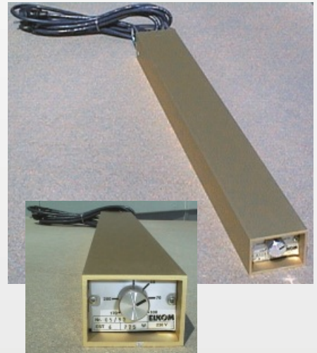
ELKOM Electrical Heating Bar EST Gold anodised aluminium profile 64x46 mm - all sides to use , compressive strength up to 200 N/cm 2 controller integrated into aluminium profile insulated temperature-adjusting knob protected against impacts or vibrations as may occur in craft establishments
