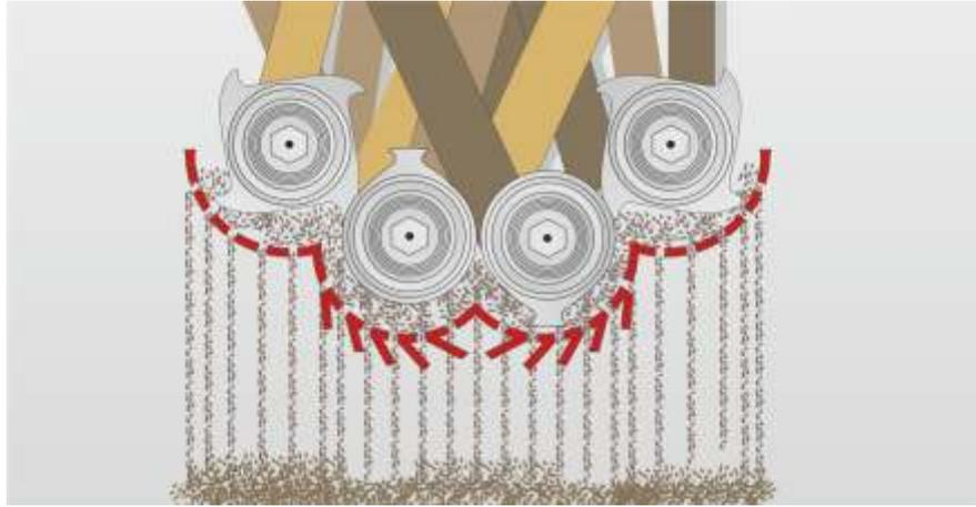
The cutting system decreed over 2 shafts with cutting blades and 2 shafts with broaching blades, as an option all shafts can be fitted with cutting blades. The cutting system is driven by firm cogwheels which run in a closed oil bath. Additional breakers underneath the perforated screen prevent the occurrence of long chips. The size of the holes in the screen determines the size of the chip.
